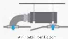
Air Intake From Bottom
